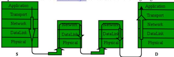
So every packet passes twice through data link layer of every intermediate router.
